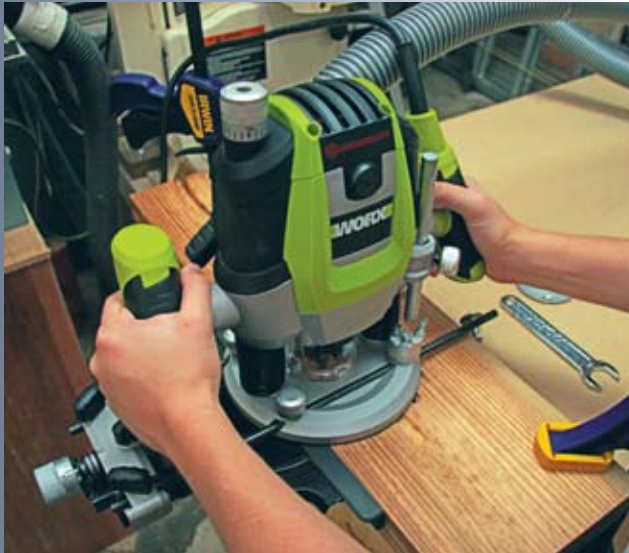
left The removable dust collection attachment makes it easy to connect the router to your shop vacuum or dust collection system
